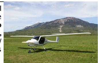
In countries which have the FAA-LSA (or adaptation of ASTM rules) categories we offer the 550 kg / 1212 lbs. MTOW version; and in countries which adhere to the UL LTF standards or similar we will make available the European Ultralight/Microlight version with the MTOW of 472.5 kg.
