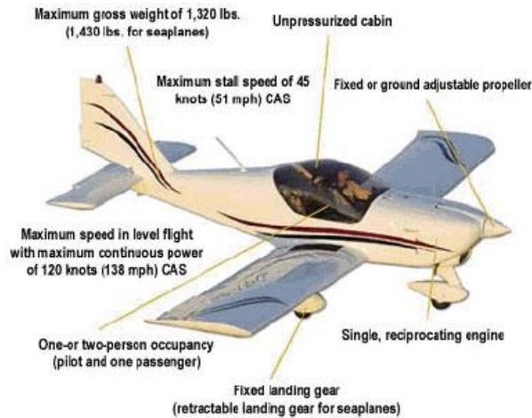
*In addition to fixed-wing airplanes as pictured, light-sport aircraft also include powered parachutes, weight-shift control aircraft, balloons, airships, gliders and gyroplanes.*
